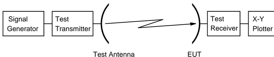
**Figure 9: Test arrangement - antenna receive pattern measurement**
